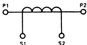
FIG. 1 SINGLE RATIO TRANSFORMER
