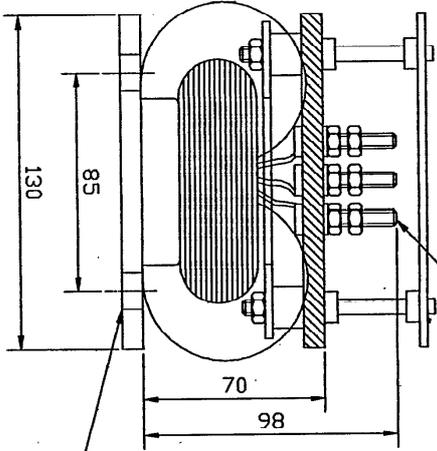
TERMINALS TO BE PROVIDED ON TOP WITH INSULATED SHROUDED COVER (M4-BRASS, TIN PLATED)
